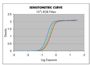
GALERIE RC DIGITAL SILVER paper exposed for 10<sup>-4</sup> seconds to broad-band colour filters illuminated by a xenon flash tube. Developer: MULTIGRADE diluted 1+9. Development: 1 minute at 20°C/68°F.
